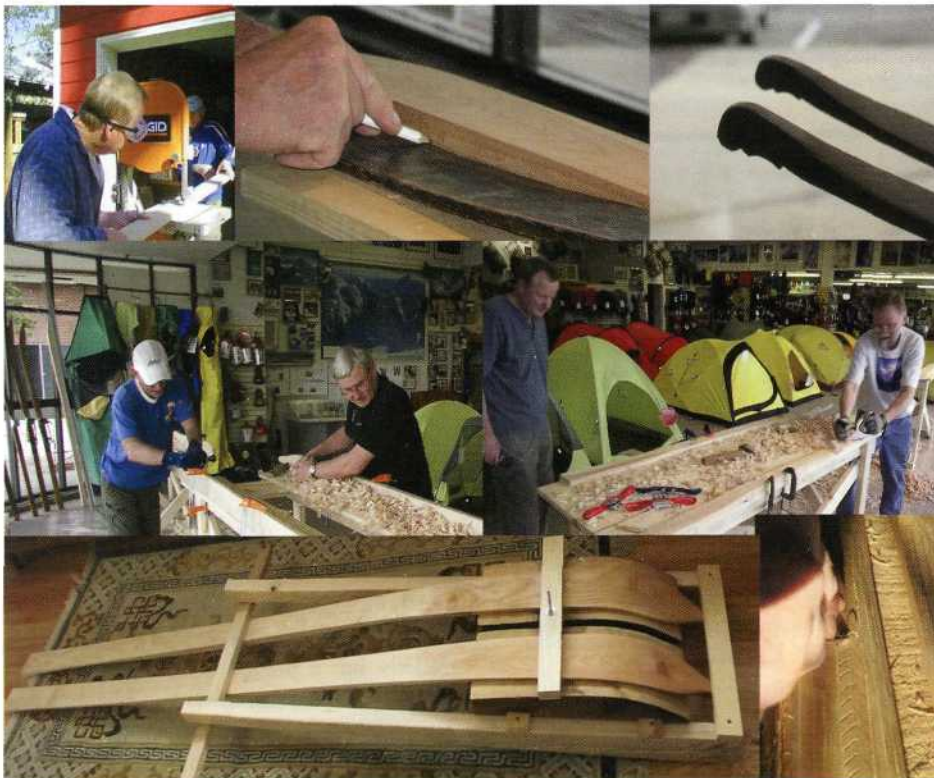
▲ 1) BOB OLSON SAWING PLANK. 2) GARY NEPTUNE MARKING SHAPE FROM MODEL. 3) CARVED SKI TIPS. 4) WAYNE BRUCKNER AND GARY NEPTUNE SHAPING SIDES. 5) BOB OLSON AND JOHN WALLACK SHAPING SURFACES. 6) SKIS IN BENDING JIG. 7) CARVING DECORATIONS WITH A PARTING TOOL. JOHN WALLACK/GARY NEPTUNE
