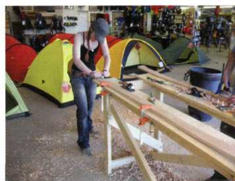
▲ ELAINE VARDEMIS IN SKI-MAKING CLASS USING A SPOKE SHAVE ON THE SURFACE. GARY NEPTUNE
